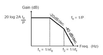
Figure 7. The frequency spectrum of the ISO 7637 surge pulses can be estimated from the rise time  $(t_r)$  and pulse duration  $(t_d)$ .
