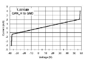
Figure 3. The current versus voltage graphs between the CAN data lines and ground show that the protection circuits are equivalent to two bidirectional Zeners with a breakdown voltage of approximately -40 V/+50 V.
