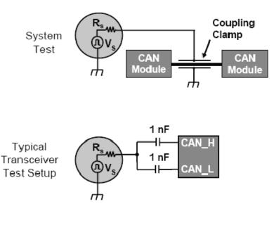
Figure 6. Surge test configurations for a system, transceiver IC and a TVS device.
