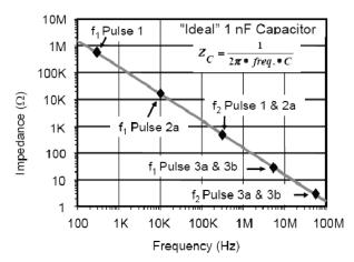
Figure 8. A 1.0 nF capacitor has significant impedance at the frequencies contained in the ISO 7637-2 pulse 1 and 2a surge tests.
