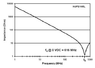
Figure 13. The NUP2105L functions as a capacitor at frequencies below the resonant frequency (f<sub>R</sub>); however, the inductance term must be included at frequencies greater than f<sub>R</sub>.
