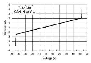
Figure 4. The current versus voltage graphs between the CAN data lines and V<sub>DD</sub> show that the transistors connected to the data lines have a breakdown voltage of approximately -40/+50 V.
