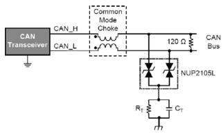
Figure 12. Adding a RC network on the ground connection of the TVS diode array increases the surge immunity by limiting the current through the NUP2105L diodes.
